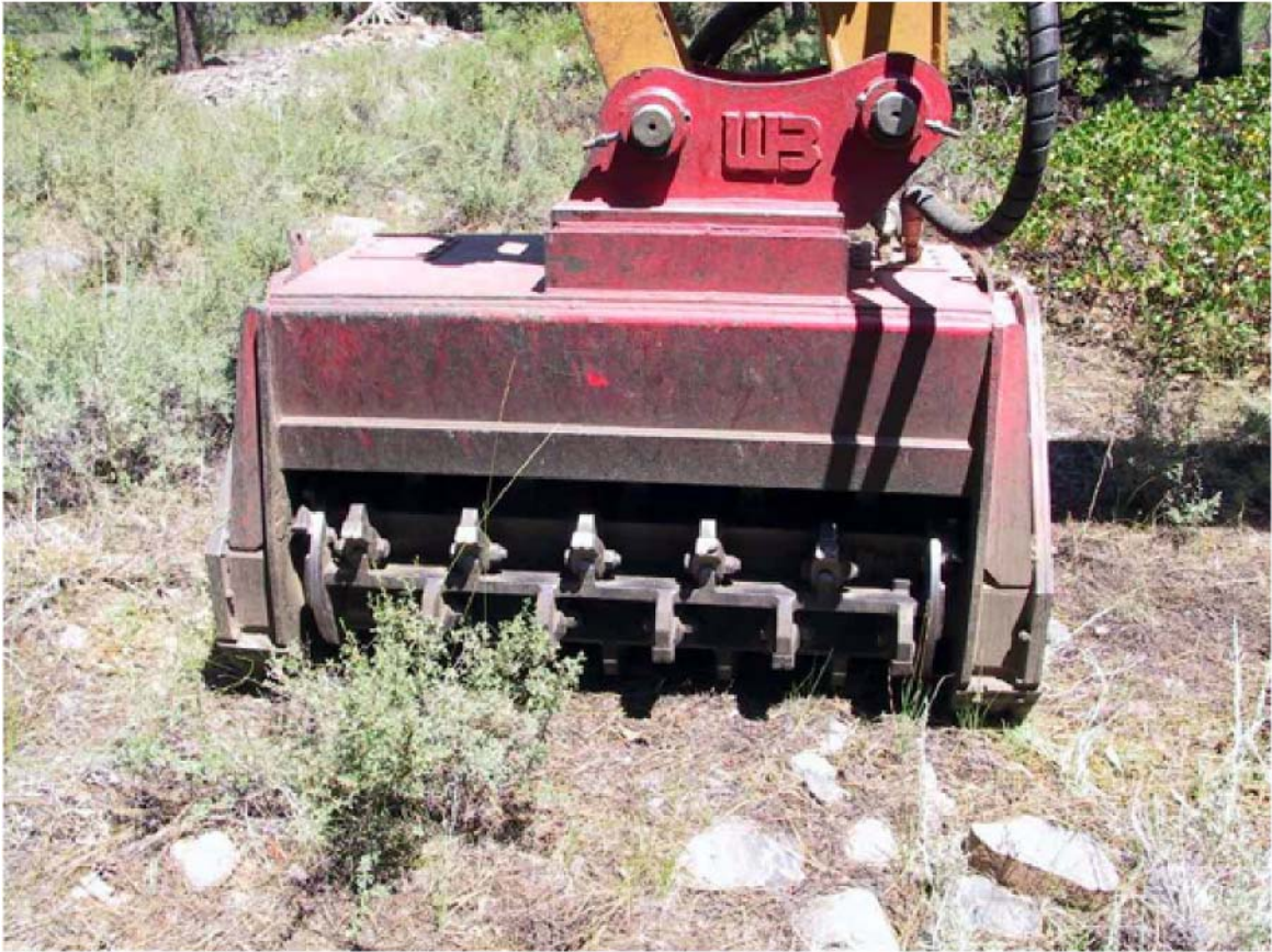
Figure 1. Fecon Bull Hog BH 80 masticator head mounted to the boom of a Caterpillar 235 excavator
